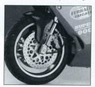
Brembo cast-iron rotors bolt directly to the front Marchesini magnesium wheel shod with Dunlop Sportmax GP-compound rubber. A special fabric weave gives the FBF carbon-fiber fender a unique striped appearance.
